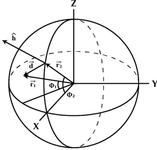
Figure 1: Vector diagram showing the geometry of the two observatories and the orientation of  $\vec{d}$  &  $\hat{h}$ .
